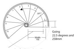
Measurement line for slope relationship between 690 and 680 measured at 7/10 of the unobstructed stair width
