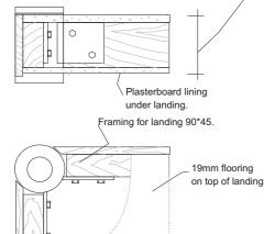
120mm overall landing thickness. If riser height is less than 180 then this dimension has to be reduced accordingly to maintain headroom 2030mm. Example with 178mm. riser it is necessary to reduce landing thickness to maximum of 100mm. In these cases we recommend the use of an enzie pre-fab landing
